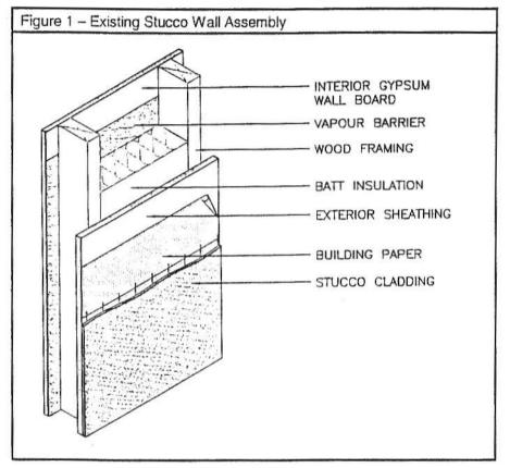
As previously discussed this wall assembly is described as "face sealed" system with a concealed moisture barrier. The combined air/vapour barrier utilizes the sealed polyethylene approach. This was typical for residential use at the time of construction. (For more information on this wall design refer to section 5.5.)
